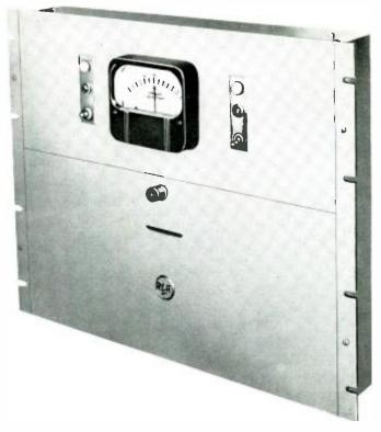
AM Frequency Monitor, BW-11A Continuous indication in magnitude and direction of any departure of carrier from its proper frequency. Wide input range of 10 mV to 25 Volts. Minimum accuracy of  $\pm 5$  Hz for one year. Provisions for remote meter or recorder.
